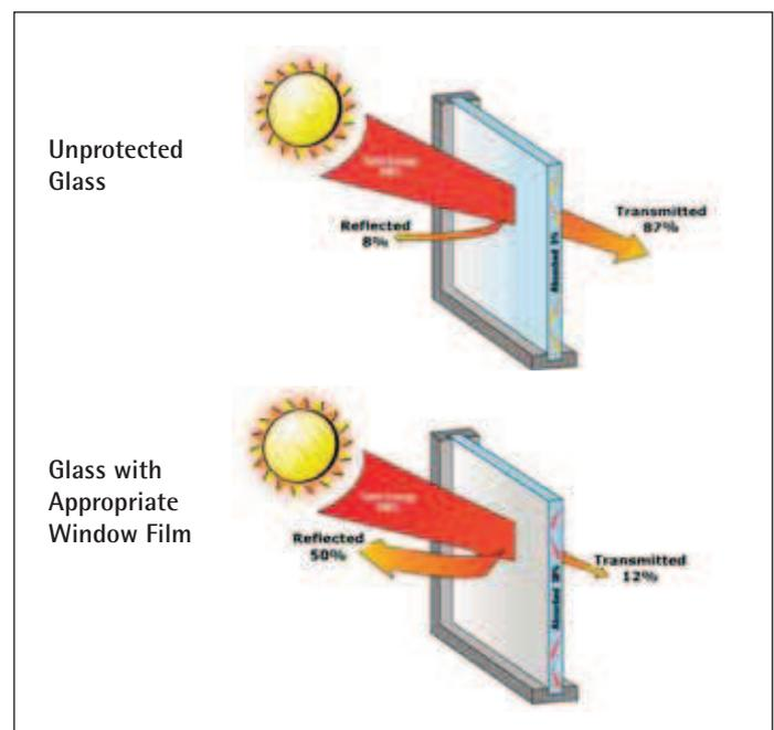
See the difference in Solar Energy transmission when comparing clear glass and glass with appropriate window film.
